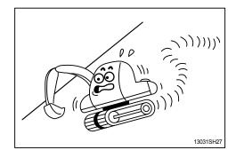
The engine angularity limits are 35 degree.
